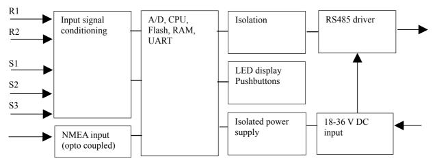
The power supply for the internal circuitry is isolated from the ship's power supply input, and the NMEA input for set-up/alignment (where needed) is opto-isolated.
