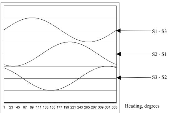
In the synchro transformer format, the angular value is transmitted using a rotating transformer with three windings, spaced 120°.
